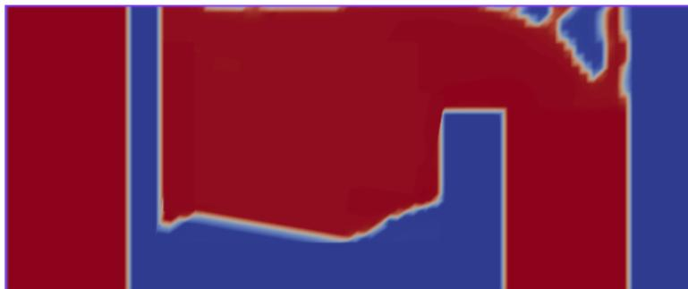
Figure 4: Thermo-magnetic optimized topology (single material). The distribution reflects a compromise between thermal dissipation and magnetic force.
