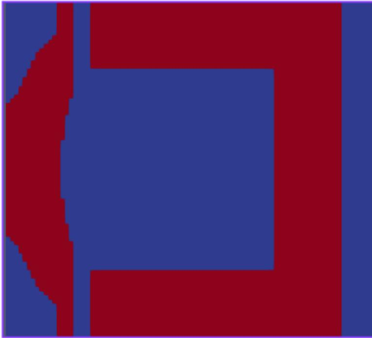
Figure 1: Optimized topology for the magnetic energy formulation. High-density regions concentrate around magnetic field gradients.
