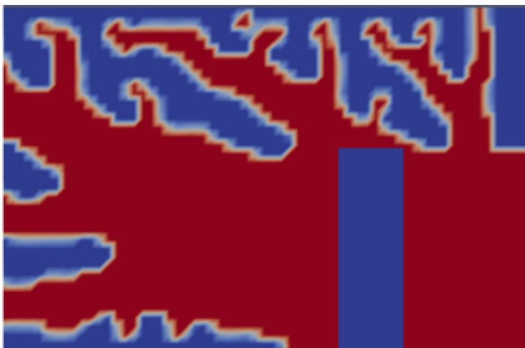
Figure 3: Optimized thermal topology. Thermally conductive material is placed to efficiently dissipate heat from critical regions.
