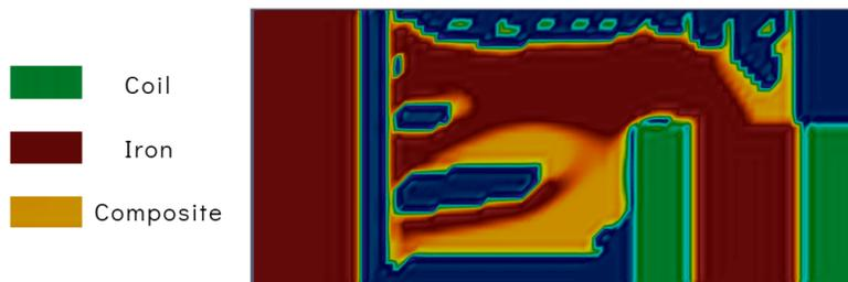
Figure 5: Multimaterial thermo-magnetic optimized topology. The solver autonomously assigns different materials to maximize performance.
