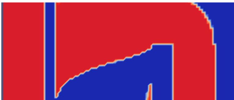
Figure 2: Optimized topology for the magnetic force formulation. Material is redistributed to maximize the force applied to the armature.
